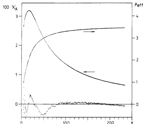
**Figure 3.** Temperature dependence of the magnetic susceptibility per chromium (left scale, cgs units) and effective magnetic moment (right scale, Bohr magnetons) of  $[(\text{tmhd})_2\text{Cr}(\text{OCH}_3)_2]$ . The lower, almost random distribution of dots around the abscissa is  $(\chi_{\text{obsd}} - \chi_{\text{calcd}}) \times 50$ , where  $\chi_{\text{calcd}}$  is based on the parameters in the text.
